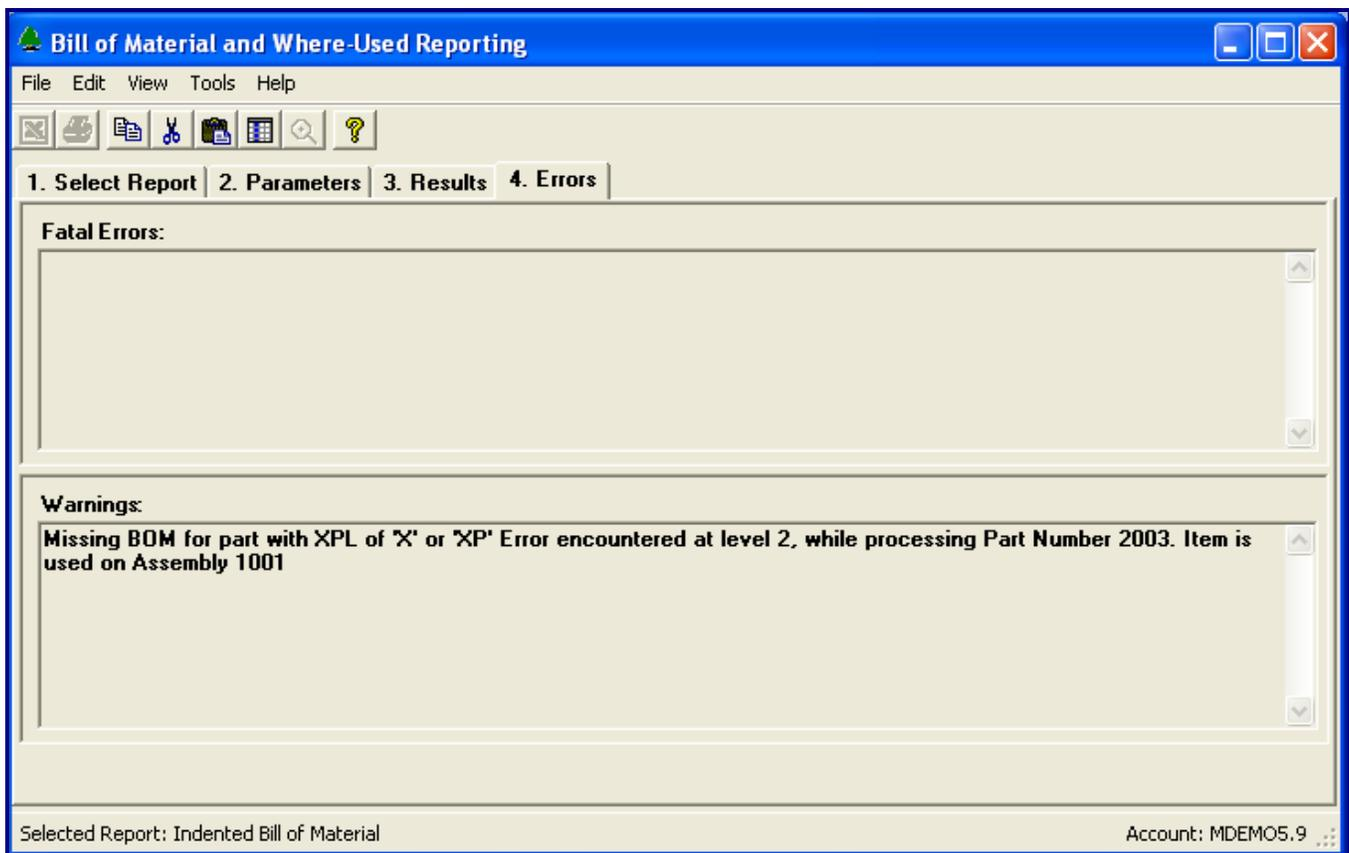
A “fatal” error means the Bill of Material could not be exploded successfully. An example of a “fatal” error would be a Bill of Material that calls itself (endless loop). In the example above, a warning is displayed when a part defined as an assembly does not have a Bill of Material.
